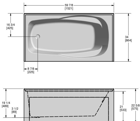
Measurement tolerances  $\pm 1/4"$  (6.3mm)
